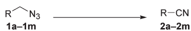
Scheme 3. Scope of the Ru(OH) x /Al 2 O 3 -Catalyzed Transformation of Primary Azides to Nitriles b
